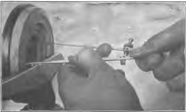
Fig. 263. Using Inside Calipers.
